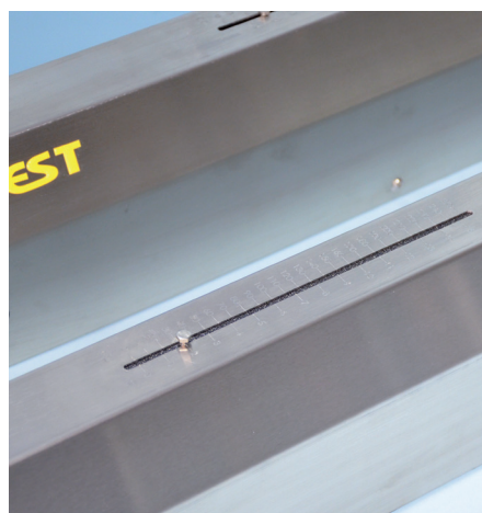
Graduated scale for approximate volume change indication
